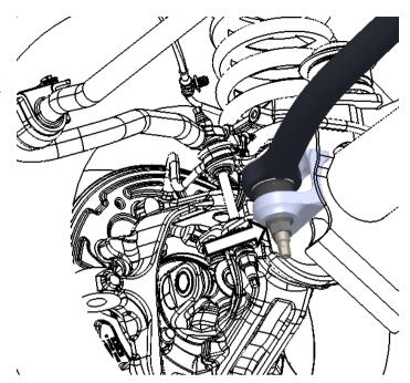
With the vehicle weight still supported by the jack stands, torque the passenger side ball joint connection to 184 lb-ft.
