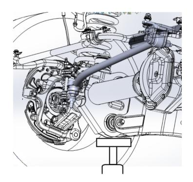
Position a jack stand under both sides of the front axle. Lower the vehicle until the front axle is supporting the vehicles weight.
