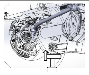
Remove the track bar-to-frame nut and bolt to disconnect the driver's side of the track bar (30mm socket).
