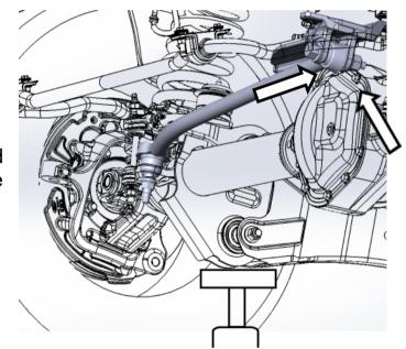
Remove nut from track bar ball joint. Disconnect the track bar from the passenger side and remove from the vehicle. (24mm socket)
