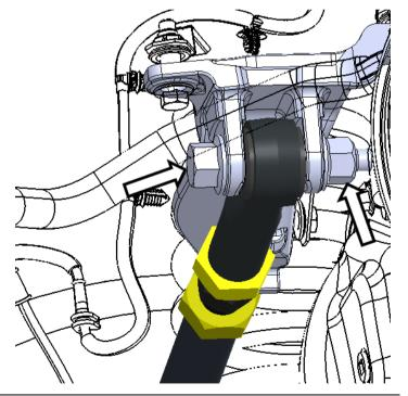
Position the passenger side of the track bar ball joint onto the frame and install supplied nut (N807659-S441) snug. (24mm socket)
