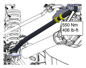
You can now perform an alignment on the front end of the vehicle. Adjust the front axle left and right by turning the threaded connector.
