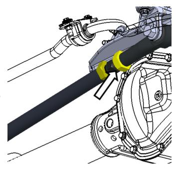
Once the alignment is complete, tighten the jam nuts to approximately 100 lb-ft of torque.
