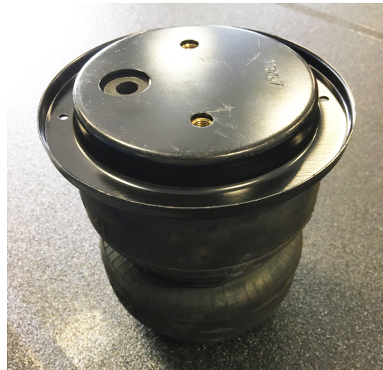
If no spacer needed (roll plate only) use the included shorter hardware Fig. 16
