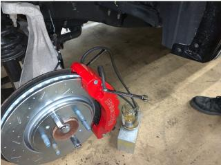
4. Open the outer bleeder screw, and let gravity fill the halves. Watch the line for several minutes and make sure that there are no more bubbles being released. When the air bubbles stop, you may close the outside bleeder. Repeat this process of the inner half of the caliper. You may need to use your hand of a rubber mallet and tap the sides of the caliper.
