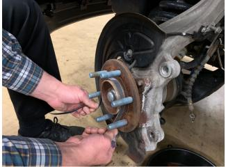
3. Place the new rotor onto the hub, and use some lug nuts to hold the rotor in place.
