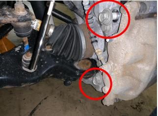
4. Using a drain pan of your choosing, place the caliper over it and remove the banjo bolt to the caliper. Allow the brake fluid to drain into the pan. There should be no more fluid coming from the brake line, as it is clamped off. This is important as you do not want the master cylinder to empty out of brake fluid.
