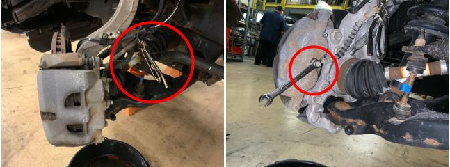
3. Using the 21mm socket, loosen and remove the M16x2.0 caliper bracket bolts. Place off to the side as you will reuse these bolts to mount the B8 caliper to the spindle. Be careful as the brake line should still be attached.
