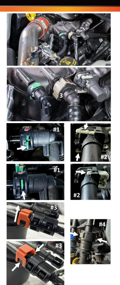
**STEP 3:** With the lines completely disconnected and clear of the fuel filter, remove the filter from the mounting canister by rotating it counterclockwise and lifting it upward.
