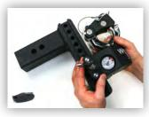
Insert the Steel Dual Pin Key Lock Assembly (F) into the Slider and lock in place by turning the key. Pull on the lock to ensure that it is engaged and place the Dust Lock Cover (E) over the lock. Do not operate without making sure the lock is securely locked in place.
