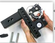
Place the Steel Weigh Safe Slider at the desired drop on the Steel Draw Bar (D) to ensure your vehicle and trailer are properly positioned. Draw bar MUST be used in the DROP position when using this pintle attachment.
