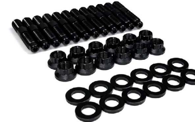
EXHAUST MANIFOLD STUD KIT XD530 // 1994-2018 DODGE RAM 5.9L/6.7L DIESEL » Black oxide coated » Higher clamping force » Allen head for easy thread-in installation » Includes (12) Studs, (12) Washers & (12) 12-Point Nuts
